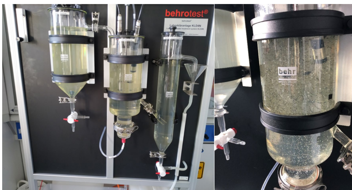
Fig. 2 Laboratory wastewater treatment plant type KLD4N/SR
