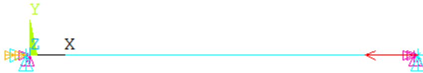
Fig. 5.3: Model of the isolated strut: cyan triangles indicate translational restrictions, orange triangles signify rotational restrictions, and pink triangles denote constraint equations between nodes due to rigid regions.
