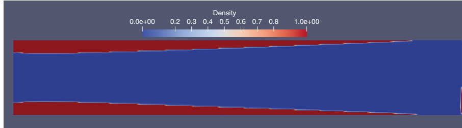
(a) Result for a domain filled with bcc unit-cells, with volume fraction \chi varying from 2% to 20%.
