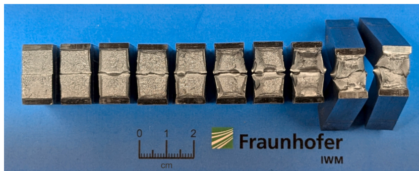
Fig. 5. Tested Charpy-V notch weld material specimens with an increase in measured total impact energy from left to right.
