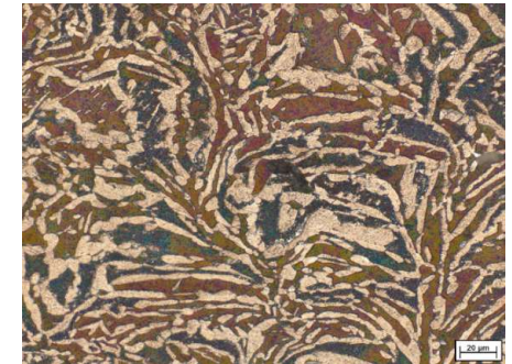
LOM: heat treated PBF (1h, 1120°C) PBF, \alpha : 53%, \gamma : 47%
