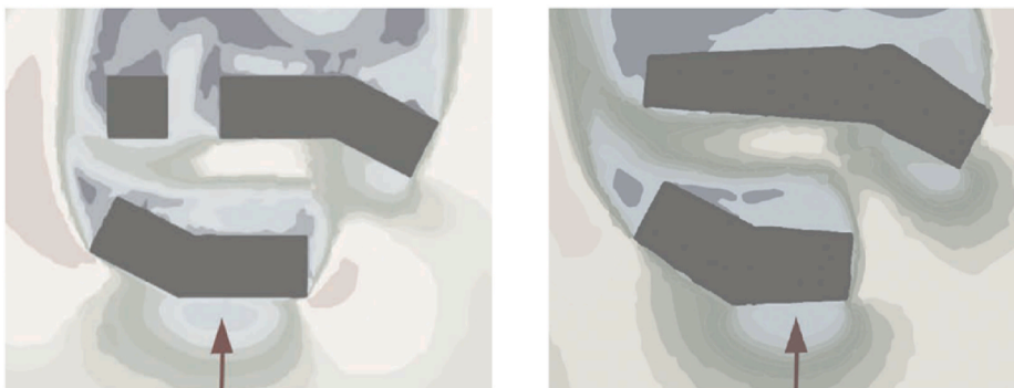
Fig. 14. CFD simulations for design 1d and 1e. The arrow indicates the direction of wind. Spacing is arranged such that there is ventilation in the courtyard to reduce heat-island effects, and at the same time reduced speed to ensure comfort.
