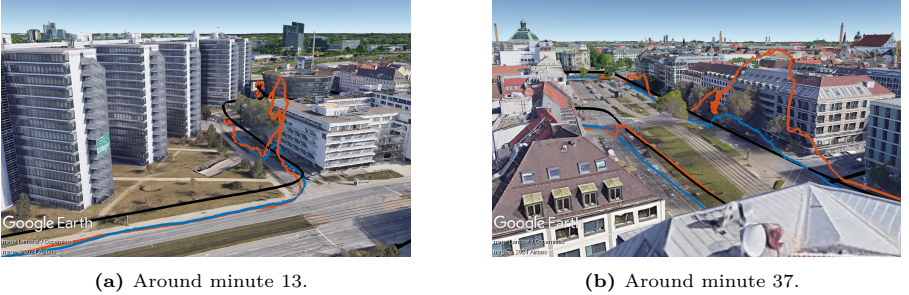
Figure 6.20: Representation of the position estimates of the urban measurement campaign in 3D renderings from Google Earth. The blue line shows the results with the VT MMEKF and the red one with the VDFLL. The black line is the ground truth trajectory. The static multipaths while stopping next to multi-story buildings lead to position errors.
