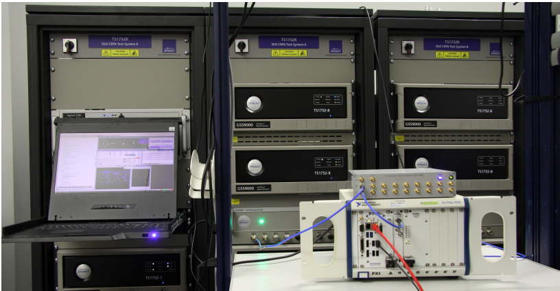
Figure 6.2: Setup for the hardware emulations. The racks of the Spirent GSS9000 series can be seen in the background. The generated RF signal is fed through the blue cable to the RF front end which sits on top of the digitizer with the NI PXIe-51740 4-channel oscilloscope card, i.e., the white machine on the bottom right.
