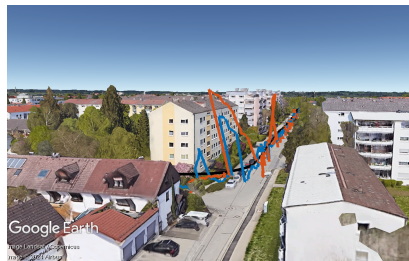
(c) Suburban section with NLOS reception around the corner.
