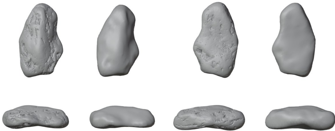
Figure 5.4. Comparison of the original grain geometry to the smoothed version (shown in shade smooth mode) after applying the Remesh modifier in Blender. In this specific case, the surface area decreased by approximately 18.25% after smoothing, while the volume only reduced by about 1.23%. However, for most cases with less extreme surface irregularities, the surface area decreased within 10%, and the volume decreased by less than 1%.
