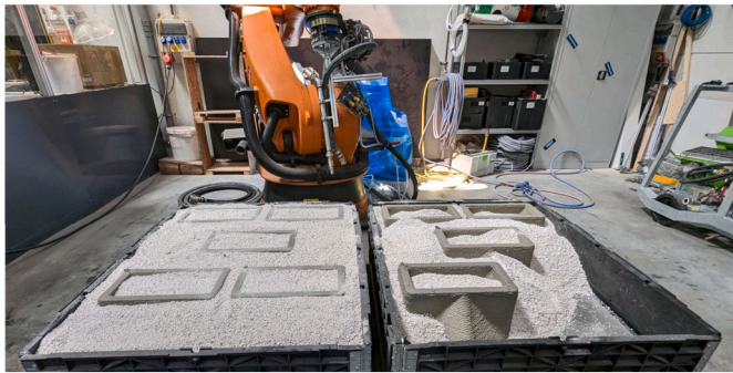
Fig. 14. Print setup with robot, nozzle in the background and print base in front with 9 pre-printed topological interlocking blocks.
