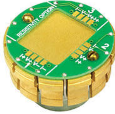
Figure 3.10.: The PPMS sample puck used for resistivity measurements. The puck features four contacts per bridge board channel, allowing for current and voltage measurements in the van-der-Pauw geometry.
