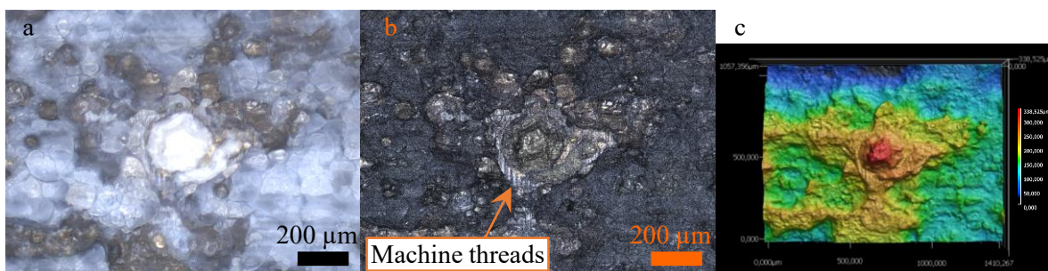
Figure F.3.: Morphological analysis of area around accumulated corrosion products on an uncoated WE43 specimen after 14 days immersion in DMEM: (a) optical microscope image, (b) topographical profile, (c) laser microscopical image.
