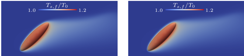
(a) Stationary ellipsoid with coupled boundary conditions in uniform flow. (b) Moving ellipsoid with coupled boundary conditions in a quiescent flow field.
