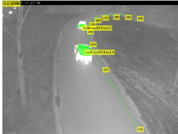
Figure 4.7: Snapshot of thermal camera 3 with the x-axis of the road coordinate system (green line with yellow labels) and the detected vehicle positions and speeds (green shapes with yellow labels)
