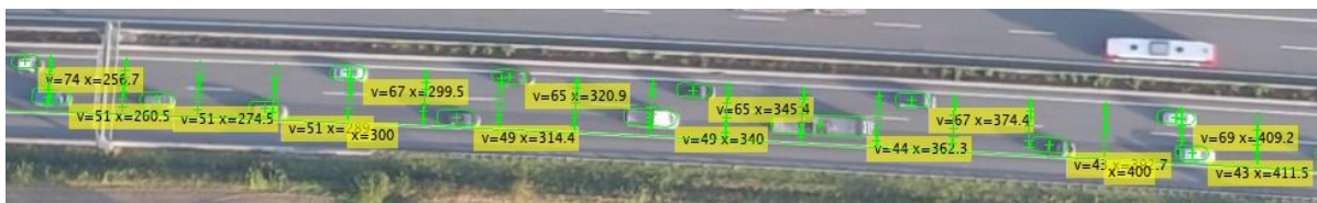
Figure 5.3: Snapshot of a drone video with vehicle detections.
