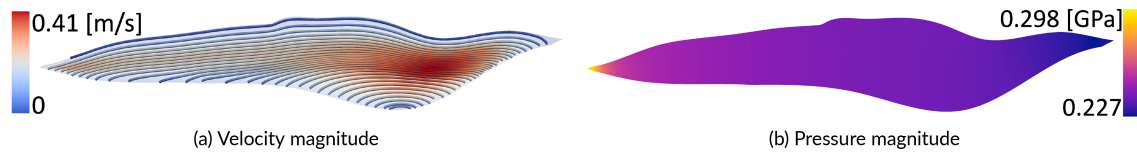
FIGURE 5 | Fluid field under boundary conditions at 675^{\circ}\text{C} , 22.5\text{ m min}^{-1} and 300\text{ MPa} after 2.5 \times 10^{-7}\text{ s} . The full domain is shown in Figure 4e.
