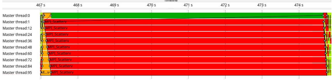
Figure 3: Vampir trace visualization of one exemplary ml_step execution highlighting the load imbalance between CPU and GPU during offloaded TBL-Transformer inference. The client processes 1 to 95 execute the same code, but only 9 of them are shown in the timeline. The pre- and post-processing is barely visible at the beginning and end of the trace. The gatherInputData() and scatterOutputData() step is highlighted in orange and red, respectively. The GPU-accelerated inference of the TBL-Transformer is highlighted in dark green on server process 0 taking more than 7 seconds of runtime.
