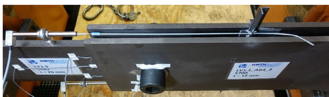
Fig. 15 Test setup, specimen LV_1.5 made of S690QL
