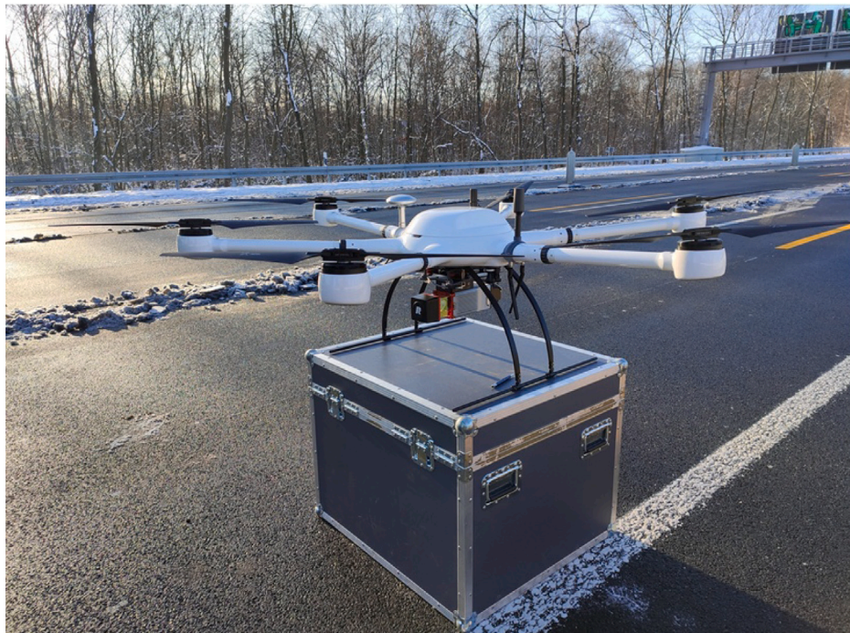
Fig. 12. Riegl miniVUX 3 UAV Scanner and drone used for surveys.
