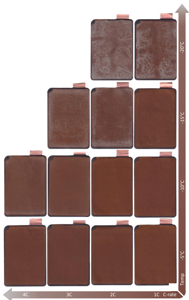
Fig. 3. Experimental condition matrix (temperature–C-rate) with representative anode scans. Representative post-mortem anode surface scans are arranged by charging C-rate (1–4C) and temperature (–5°C to –20°C), defining the experimental design used throughout the manuscript. At the most extreme low-temperature/high-C-rate combinations, charging terminated early due to voltage limits, so no sample is available. (For interpretation of the references to color in this figure legend, the reader is referred to the web version of this article.)
