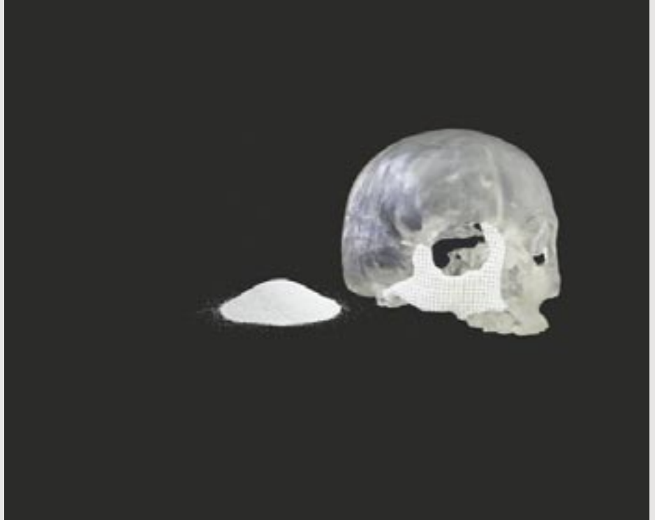
Bild 4: Lasergesintertes Schädelimplantat [RKW+08]. Quelle: Rietzel, D., Kühnlein, F., Wendel, B., Feulner, R., Hülder, G.: Enhanced range of plastics for Selective Laser Sintering: serving different user profiles and also consumer and industry requests. Quelle: Proceeding Euro-u Rapid 2008, Berlin, September 2008.
