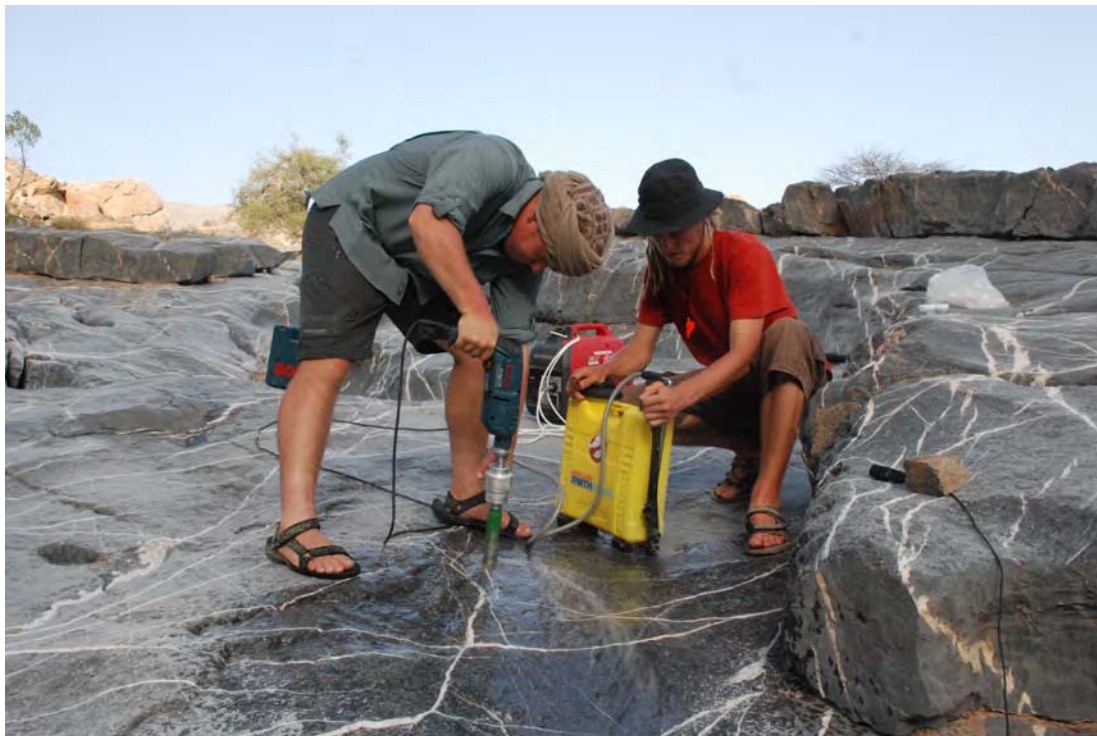
Figure 27: Taking rock plugs from the outcrop: One person operates the drilling machine while the other maintains a steady flow of cooling water with the pump. The generator in the background provides the electricity.
