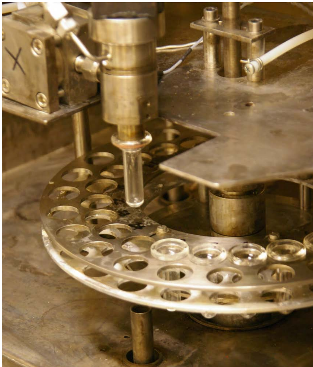
Figure 33: Look into the Kiel device. The thimbles are placed in a carousel. For reaction and measurement they get picked up with a vacuum plunger. The Kiel device is partly located inside an oven that maintains a constant temperature of 90° C.
