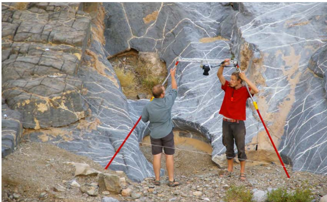
Figure 9: Assembly of the photography setup. The camera is pointing vertically downward. In the pictures the telescopic legs are locked in the second position.
