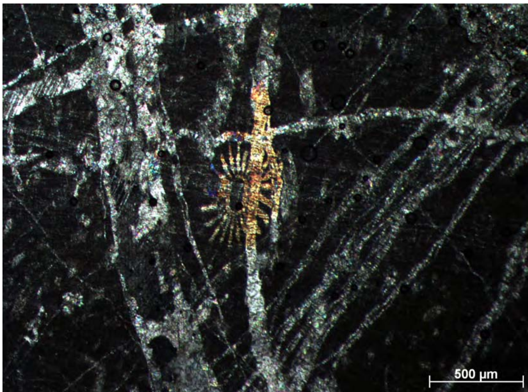
Figure 50: Figure shows lateral crystal growth not only in cross cutting veins (upper image), but also occurring at crossed cut Quartz fossils (lower image). Both images are taken under crossed polarized light.
