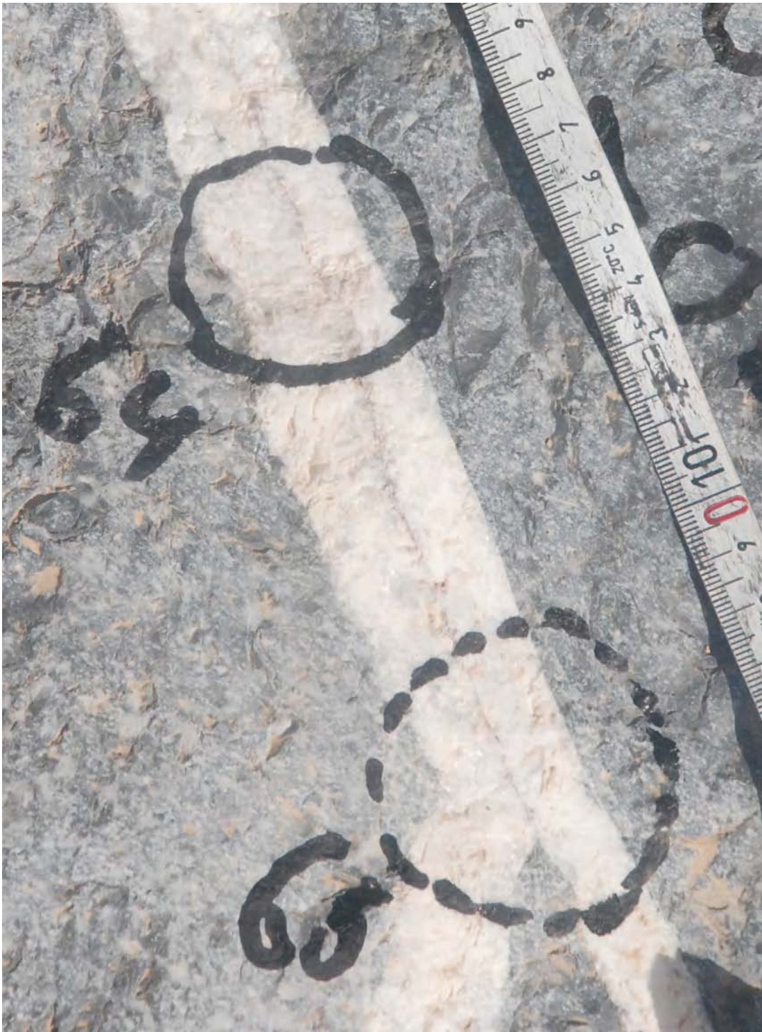
Figure 25: a North south striking vein aligns a 131^\circ striking vein, forming a stack of veins. The aperture of the stack is approximately the sum of the aperture of the single veins and the boundary between the veins stays distinguishable in the stack.
