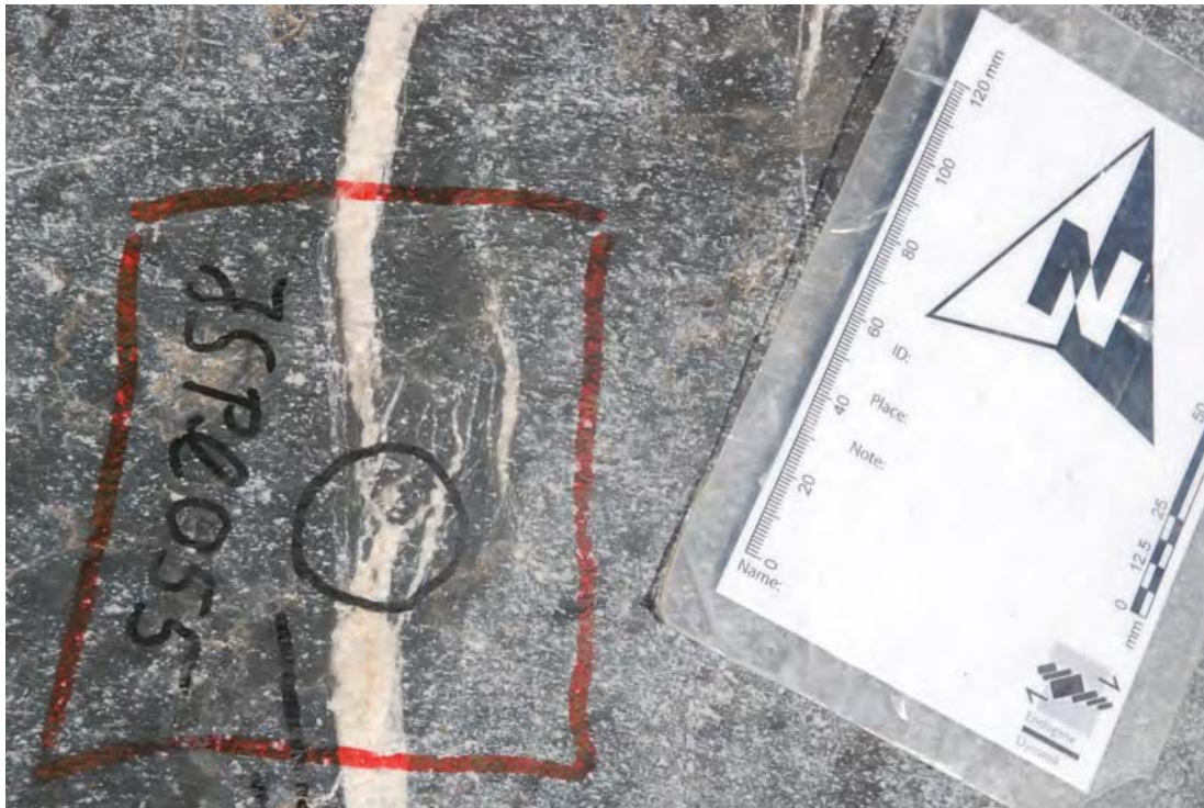
Figure 24: example for a splay within a vein. The vein splits up into several smaller veins but then proceeds with unchanged aperture and strike direction (here: 10 mm, 156°). Splays in which veins terminate are called tip splays.
