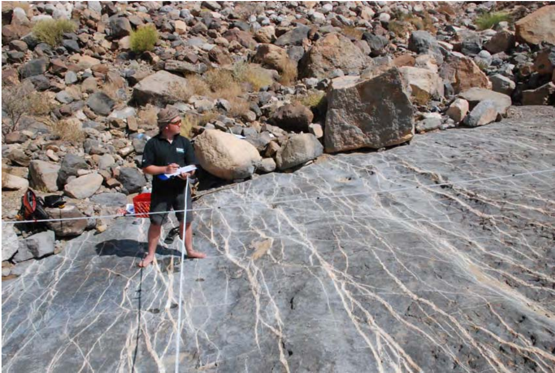
Figure 10: As the first step the 2 orthogonal axes of the grid are established with measure tapes and carefully beared.
