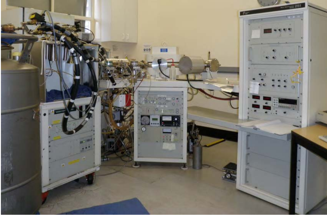
Figure 29: Photo of the mass spectrometer lab. The Kiel device is located in the left of the picture. The electronics of the mass spectrometer are located in the cabinet on the right. You can see the mass spectrometer in the middle of the photo. (Photo courtesy: Paul Stenhouse)
