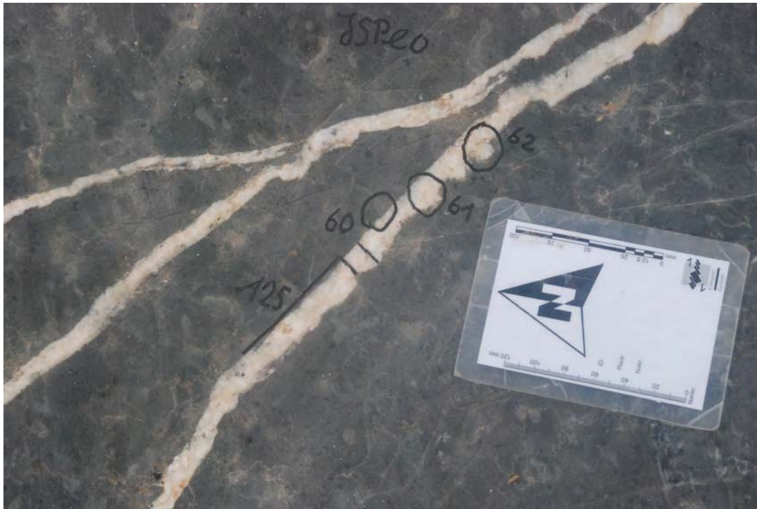
Figure 26: the highly lobate shape of the southern vein/host rock interface of this 125° striking vein gives it the attribute of a “chainsaw” vein. In this case only one wall of the vein shows a chainsaw pattern. At some veins it also appears on both vein/host rock interfaces.
