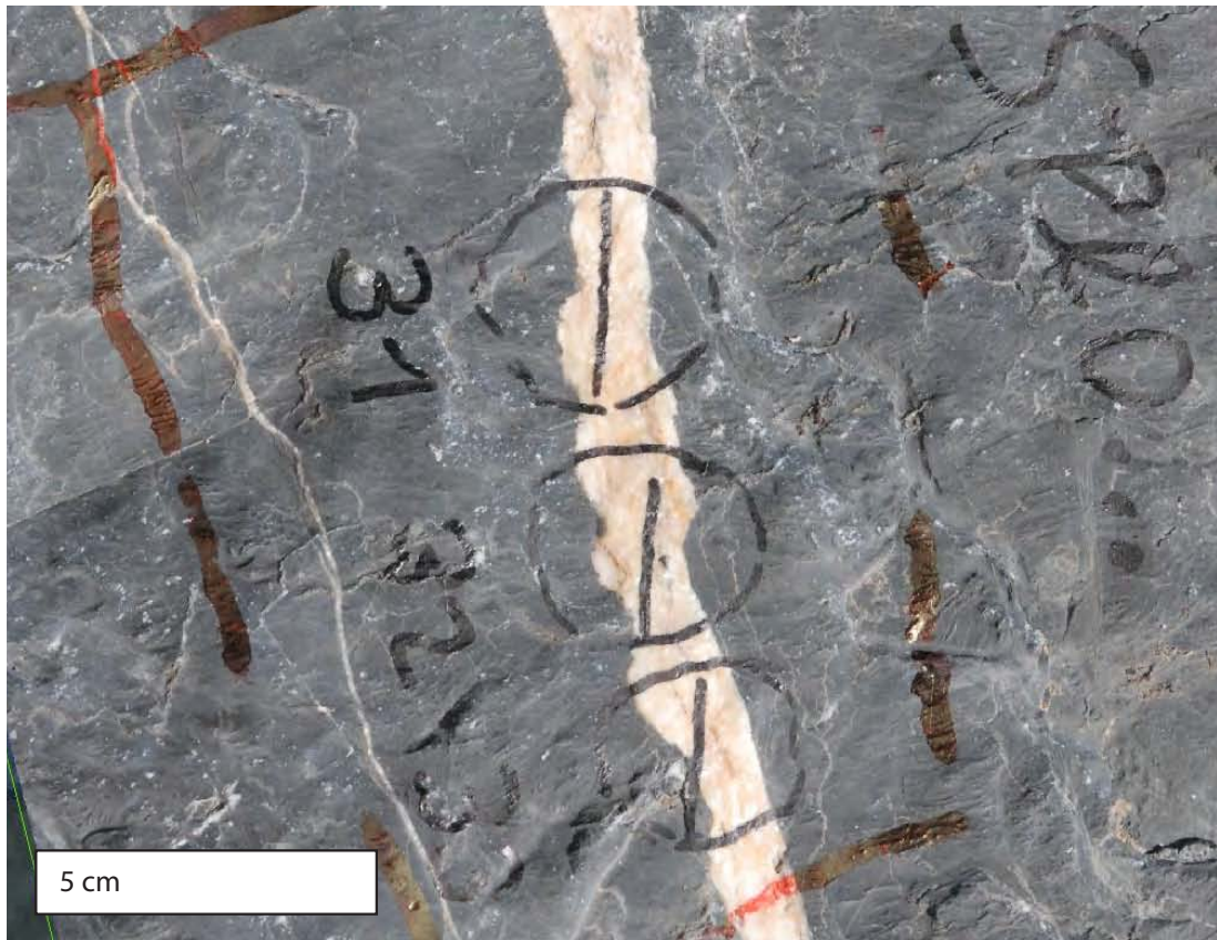
Figure 45: The image shows a site of planned plug samples (JS-PL-031,32&33) to investigate the chainsaw structures visible on the detail image. The left vein-host rock interface is undulating while the right one does not show this behavior.
