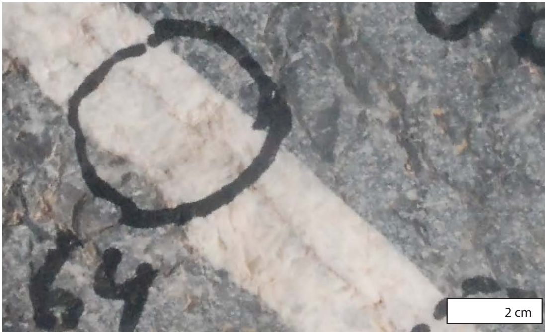
Figure 43: The figure shows a planned plug samples site (JS-PL-064). The vein's texture can be roughly seen to appear blocky with grain sizes up to 1 mm.
