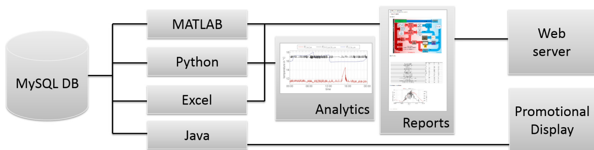
Figure 4.10: Schematic of the data access and processing system with online publication
