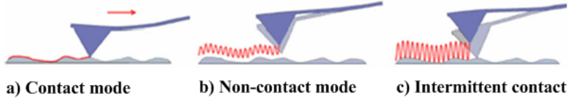
Figure 2.2: Modes of operation: contact mode (A), non-contact mode (B), and intermittent contact (C). In contact mode the tip is scanned across the surface, the cantilever being deflected as it closely follows the surface topography. In non-contact mode a stiff cantilever is oscillated in the vicinity of the sample, while the sample is raster scanned. In picture C the tip taps the sample during each oscillation and it is restored to the original position at the end of each cycle, operation called intermittent contact [14].
