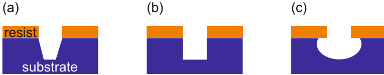
Figure 3.6: Etch characteristics: sputtering (a), physically assisted chemical etching (b), chemical etching (c)
