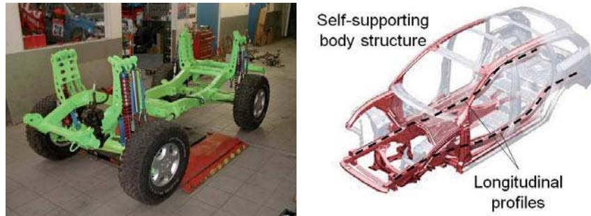
Body on frame of Mercedes G [4] Body integrated frame - Audi Q7 [8]
