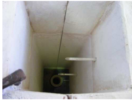
Fig. 5.2: Thermal couples in the casting mould, top view
