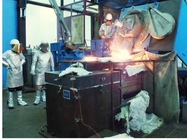
Fig. 5.10: Casting of the 500 kg ingot at IEHK, direct tapping and use of a runner
