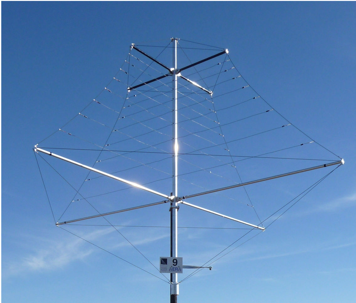
Figure 8.1: Photograph of the Small Black Spider LPDA installed at AERA.
