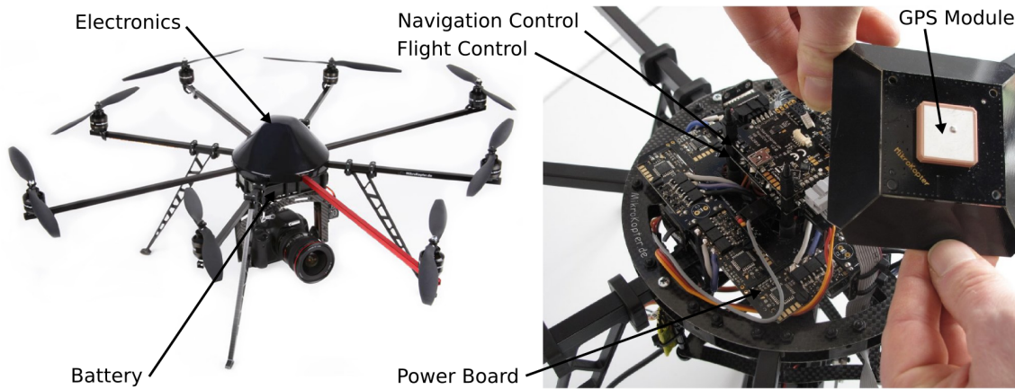
Figure 9.4: Photograph of the 'Mikrocopter Okto XL' prepared for aerial photography. On the right picture the center with the electronics boards is shown. Photographs from [181].
