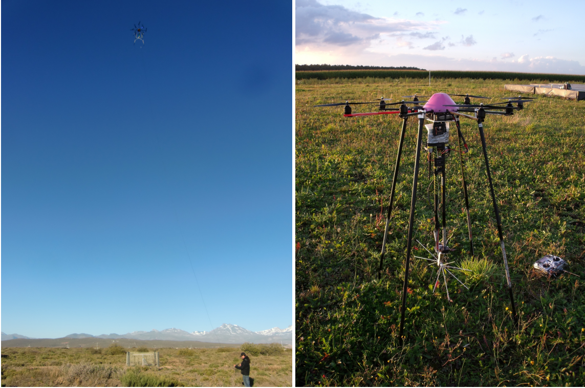
Figure 9.5: Photograph of the octocopter calibration setup at the AERA site with the octocopter hovering in about 30 m height above an AERA phase 2 station equipped with a Butterfly antenna (left). On the right the octocopter with attached transmitting antenna and prepared with an additional differential GPS for test measurements at the LOFAR radio detector in the Netherlands is shown.
