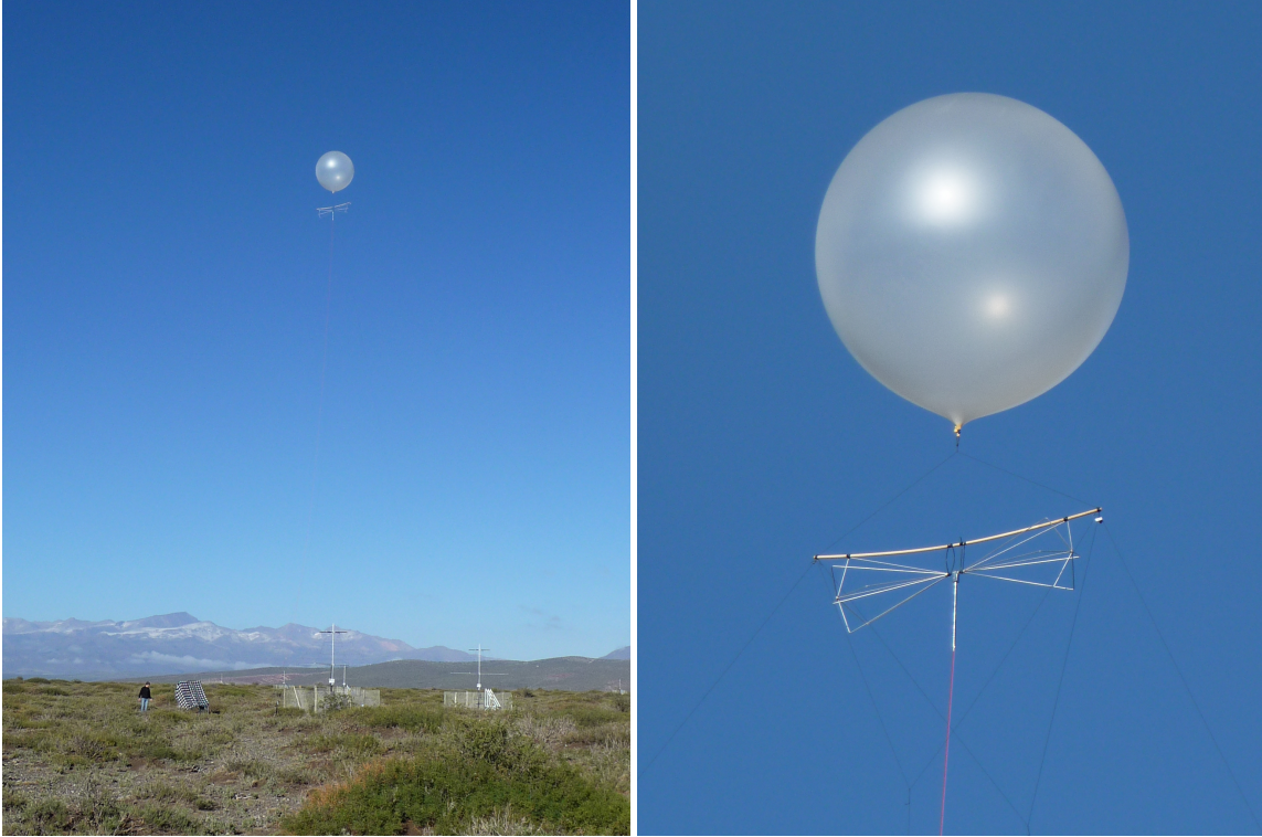
Figure 9.2: Photograph of the balloon calibration setup at the AERA site. The left photograph was taken during a calibration measurement of the SBS antenna with the balloon hovering almost in the zenith of the detector station in the foreground. On the right a zoom to the balloon with the transmitting antenna is depicted.
