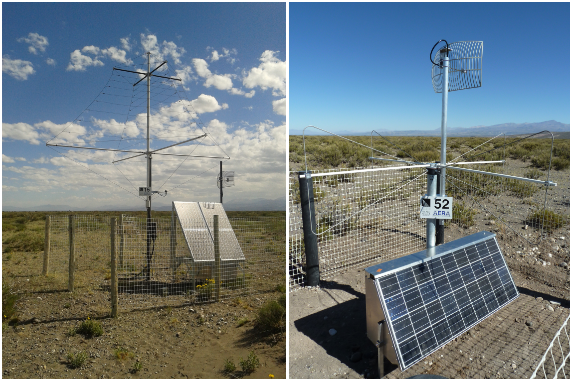
Figure 6.3: Photograph of phase 1 (left) and phase 2 (right) radio detector stations of AERA.
