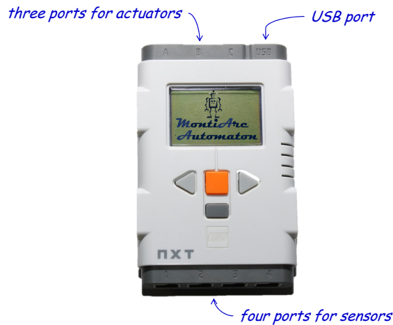
Figure 8.3.: The Lego NXT brick with a 48 MHz processor and 64 KB RAM.
