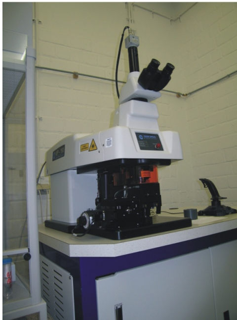
Figure 3.2, Layout of the laser ablation system developed at ETH Zürich and also used by the Institute of Mineralogy and Economic Geology at the RWTH Aachen, modified after Heinrich et al. (2003)
