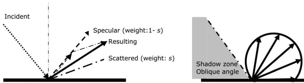
Figure 4.9 - (left) Vector based scattering as implemented by Odeon: reflecting a surface with a scattering coefficient of 0.5 results in a reflected direction which is the geometrical average of the specular direction and a random scattered direction; (right) Oblique Lambert approach produces a shadow zone (no sound is reflected), which is small for high scattering values (after Christensen, 2009).
