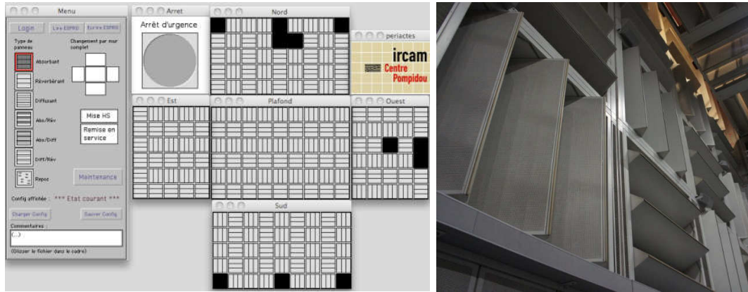
Figure 7.3 - (left) MaxMsp patch for controlling the movements of periaetes; (right) prospective view of a sidewall at ESPRO.
