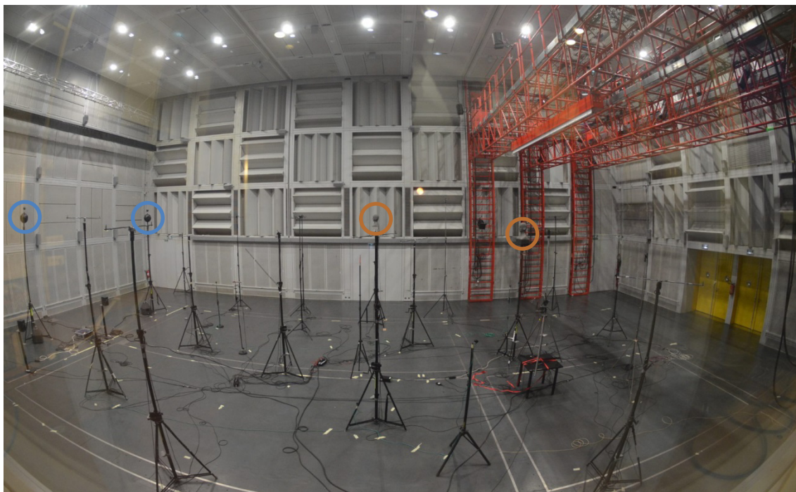
Figure 7.6 - Measurement setup inside the ESPRO during the measurement of configuration 15 (view from the control room); the 3-way loudspeakers and the two dummy-heads are highlighted in blue and orange respectively (from left to right: S1, S2, Pos. 14, Pos. 21).
