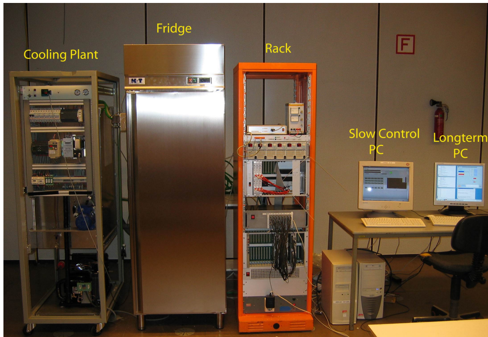
Figure 2.16: Photograph of the petal longterm test setup in Aachen. It consists of a refrigerator, where the petal is put in, a cooling plant, a rack with the electronics and two PCs, one used for the slow control and the other one for the longterm test software.
