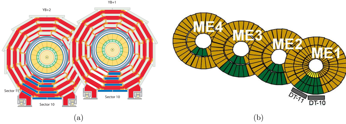
Figure 3.3: The muon detectors used in the MTCC as cosmic trigger. (a) Barrel wheels YB+1 with sector 10 and YB+2 with sectors 10 and 11 equipped with DT chambers and RPCs, covering a \phi angle of about 30^\circ and 60^\circ , respectively (in blue). (b) Muon end cap disks ME1, ME2 and ME3 partially instrumented with CSCs covering a \phi angle of about 60^\circ (in green). The detectors mounted on ME4 did not participate in the MTCC.
