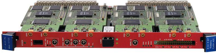
Figure 2.7: The Double Chooz wave form digitizer: CAEN model V1721 [43].
