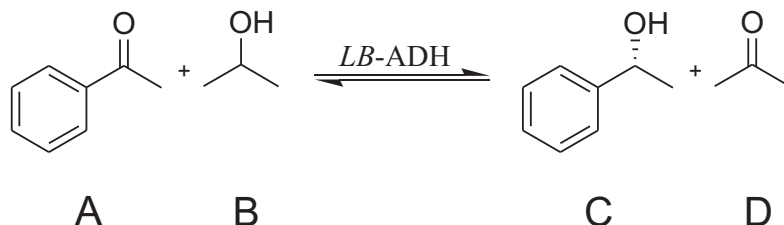
Scheme 2.1: Model reaction is the enantioselective reduction of acetophenone to ( R )-1-phenylethanol using 2-propanol and acetone; the catalyst used is LB -ADH.
