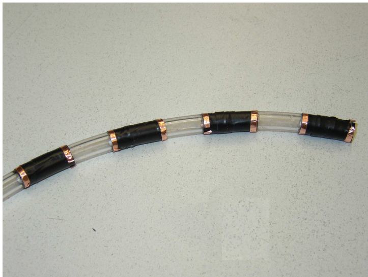
Figure 6.8: Plastic tube that mimics a vessel and that was attached to the phantom. Alternate dark bands and radio-opaque metal bands provide spatial reference.
