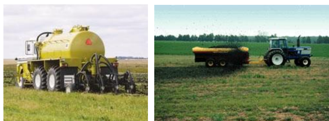
Figure 5. Tank wagon for spreading liquid sludge (left, LRRM) and tractor applying dewatered sludge (right, Fox River Watch).
