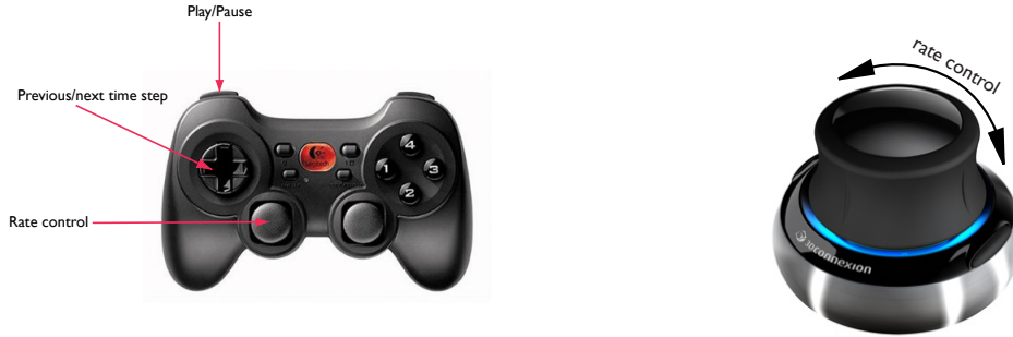
Figure 4.6.: Two examples of physical devices for time navigation. Left: The left-hand side elements of a Logitech Rumblepad™ are used for time control. Play/pause input conditions are mapped to a single, easily reachable button, one-step maneuvering target selection is mapped to a digital left-right control (one time step backwards/forward), and speed selection is mapped to one axis of an analog joystick. Right: One axis of the isometric 3Dconnexion SpaceNavigator™ is used to control speed.
