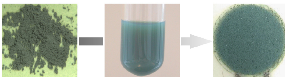
Figure 3.9: Scheme of thick film deposition and photograph of thick film.
