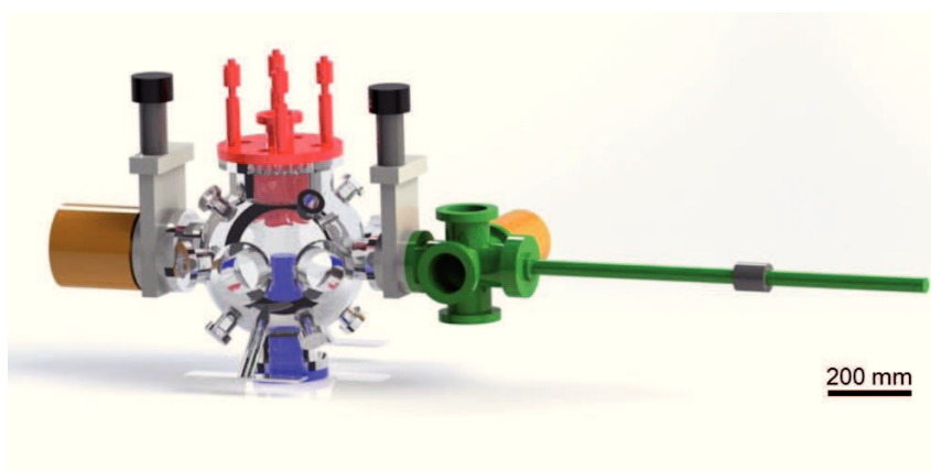
Figure 2.2: Schematic drawing of the ultra-high vacuum sputtering system used. The magnetron cluster flange, substrate holder, load lock system and turbo pumps are depicted in red, blue, green and orange, respectively.
