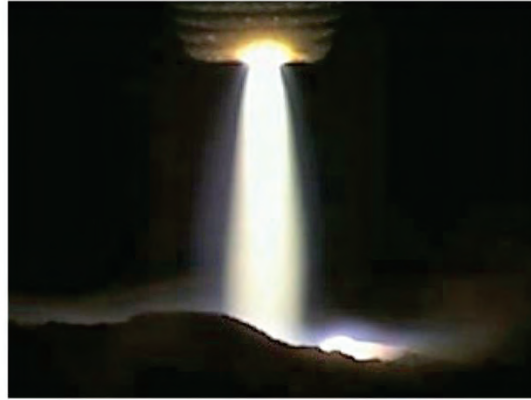
a) Arc current I_{\text{arc}} = 500 A, Arc length \ell_{\text{arc}} = 50 mm (cylindrical, steady state arc)
