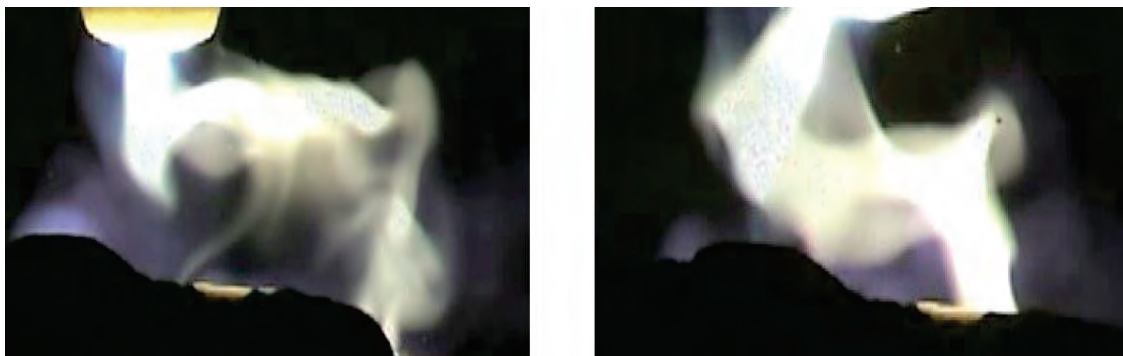
c) Arc current I_{\text{arc}} = 2000 A, Arc length \ell_{\text{arc}} = 50 mm (example frames)
