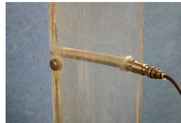
Figure 5.3.: Accelerometer sensor placed in position 4 and short rod 10.
