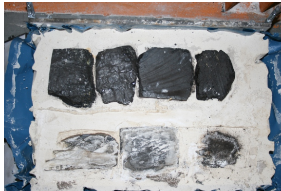
Figure 5.29.: Sample box containing two rows; coal (upper row) and dead rock (lower row) [NKBB12].
