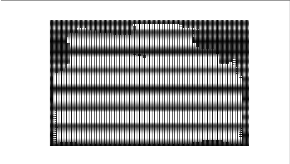
Figure 5.26: Final adapted grid, Re = 100 , lid-driven Cavity.
