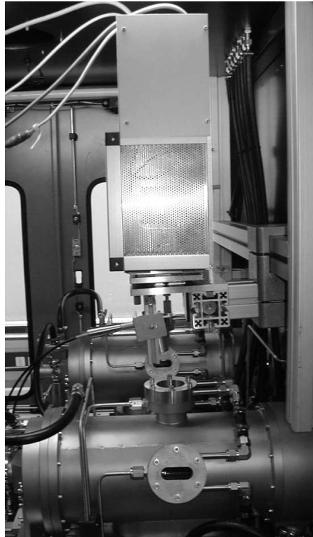
Figure 4.1: The AIX 200/4 horizontal reactor equipped with in-situ reflectometry and pyrometry (EpiR-TT)
