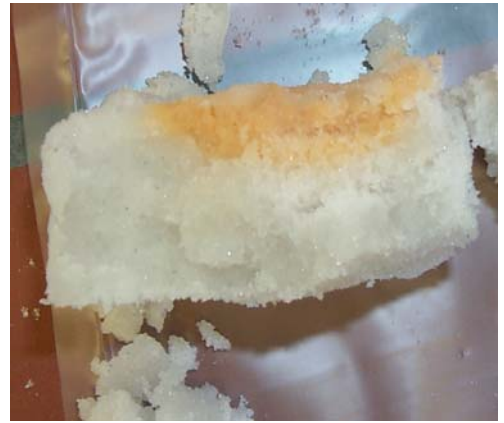
Figure 4.13. Column experiment under unsaturated conditions ( S=80\% ) with Rhodococcus rhodochrous , the sand grain size was 330\ \mu\text{m} . the sand surface close to the injection point is shown. (A). Surface of the first sand layer. (B) Transversal cut of the first slice.
