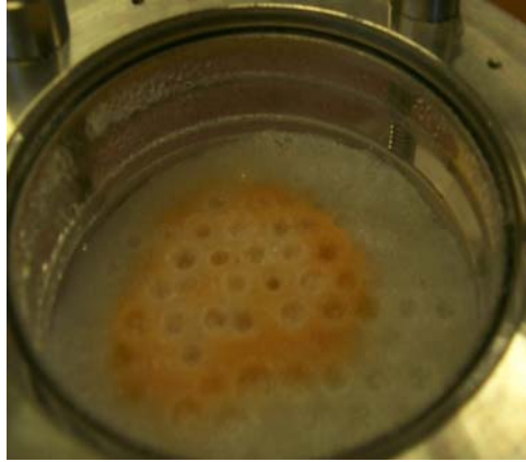
Figure 4.13. Column experiment under unsaturated conditions ( S=80\% ) with Rhodococcus rhodochrous , the sand grain size was 330\ \mu\text{m} . the sand surface close to the injection point is shown. (A). Surface of the first sand layer. (B) Transversal cut of the first slice.
