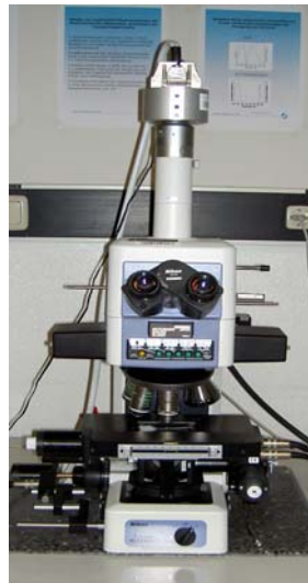
Figure A7. The epifluorescence microscope (Nikon ECLIPSE E 1000 with a motorised and PC controlled. The images were captured with a CCD camera, Sony DXC-9100 P, and a Matrox Corona Framegrabber.
