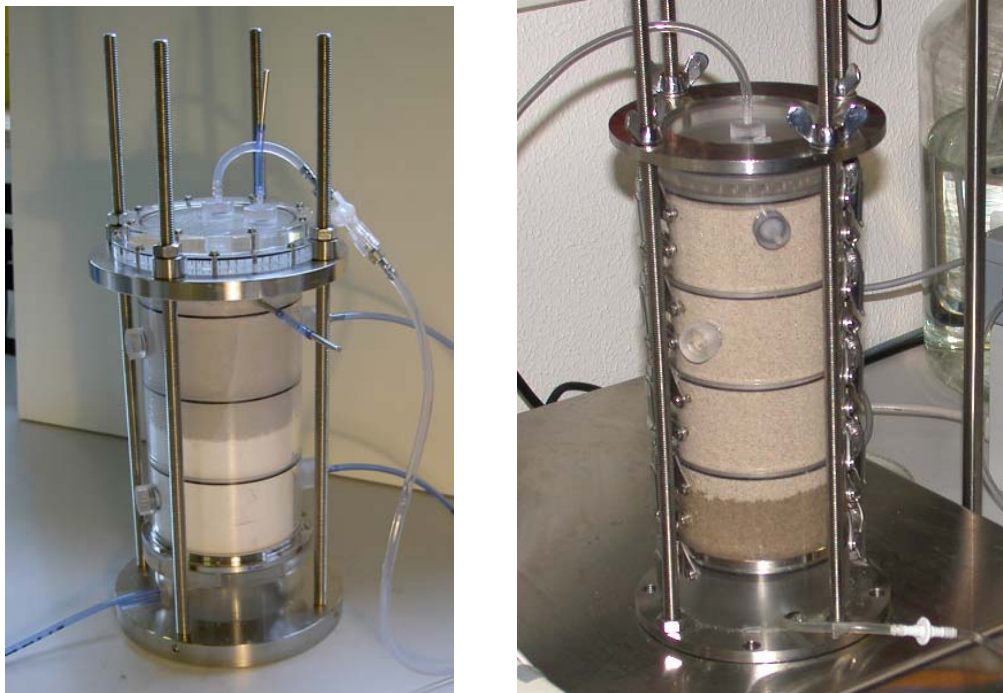
Figure 3.7. Full saturation procedure (Left): The column is emptied using a vacuum pump from the bottom and degassed water is injected from the top. Procedure to achieve 80% saturation (Right): The column filled with dry sand is successively filled with water from the bottom to the top.
