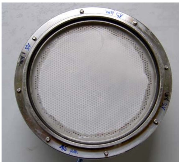
Figure 3.5. Stainless-steel plate covered with a suction membrane 15 \mu m mesh size.
