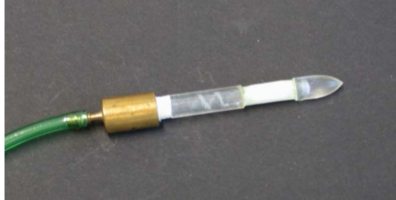
Figure A2. Tensiometer with 1 \mu\text{M} membrane.
