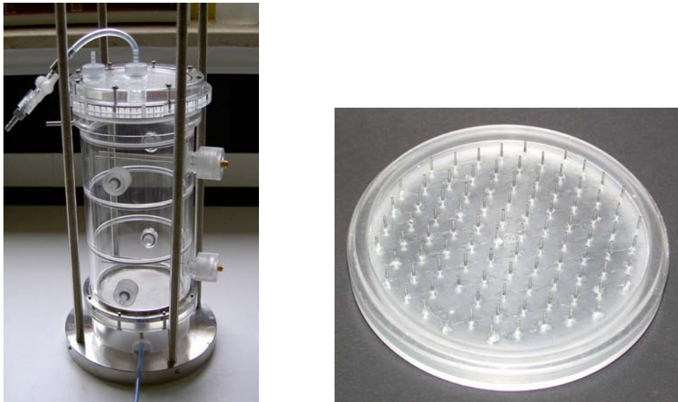
Figure 3.4. (Left) Plexiglas column. (Right) Sprinkler supplied with stainless steel needles.
