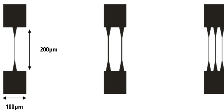
Figure B.8: Design for the Crossbar Electrodes. 100 \mu\text{m} bond pads are connected by wires. The wires have taper-triangles at both ends. The width of wires is varied between 1 \mu\text{m} and 100 nm.
