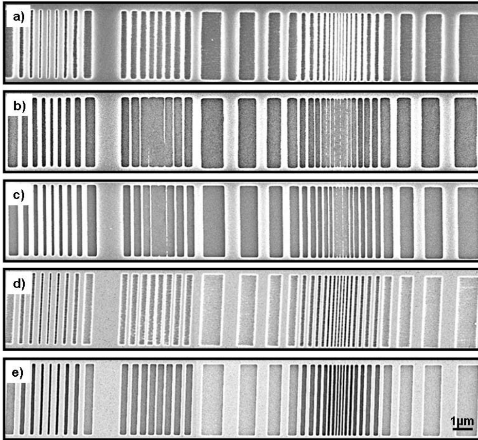
Figure 4.5: Comparison of different development recipes for PMMA masters SEM images (10kV). The height of the PMMA layer was 230 nm. a) standard development without any assistance b) development in a ultrasonic bath c) development in a 1 MHz megasonic bath at 60 % power d) development in a 2 MHz megasonic bath at 30 % power e) development in a 2 MHz megasonic bath at 100 % power
