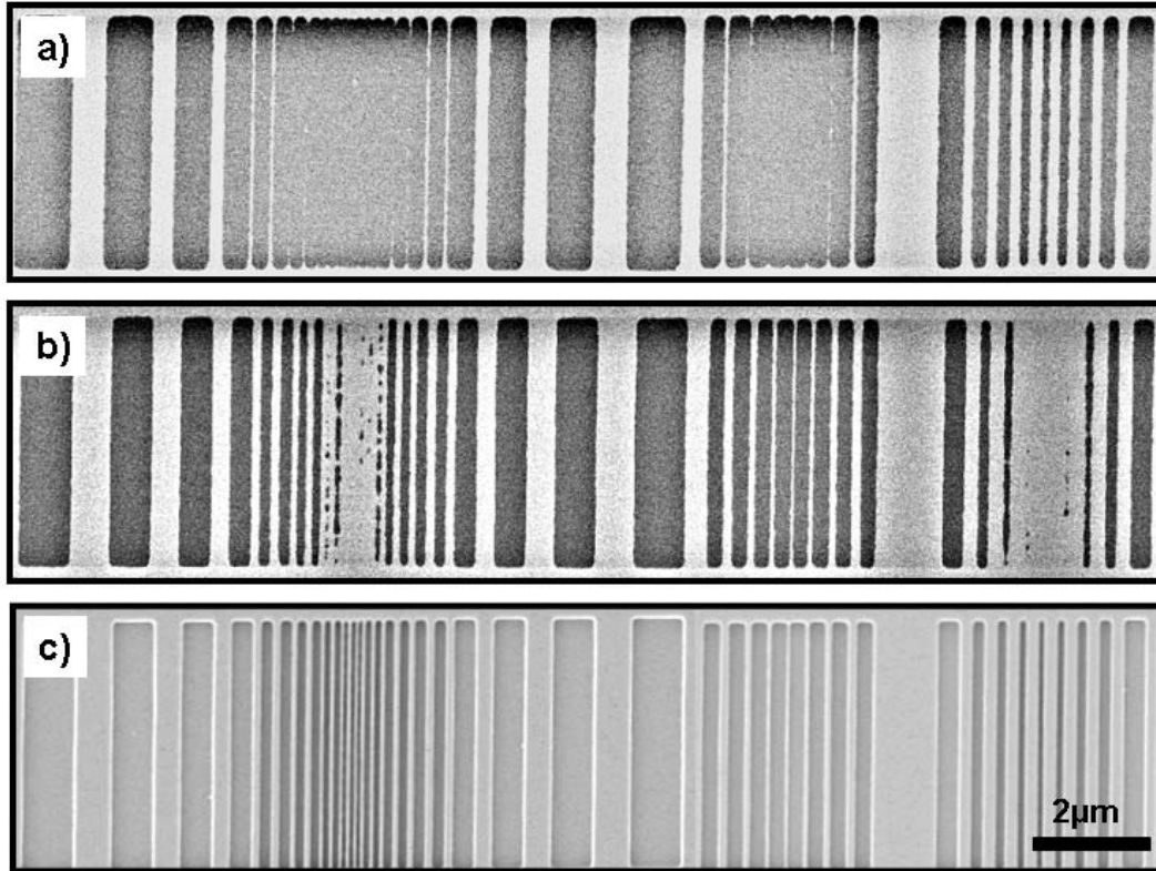
Figure 4.3: Comparison of the 75 nm design in different resists SEM images (10 kV) of a) HSQ on silicon written with a dose of 110 \mu\text{C}/\text{cm}^2 b) HSQ on silicon written with a dose of 150 \mu\text{C}/\text{cm}^2 c) PMMA on silicon written with a dose of 250 \mu\text{C}/\text{cm}^2 . The master was covered with a sputtered gold film.
