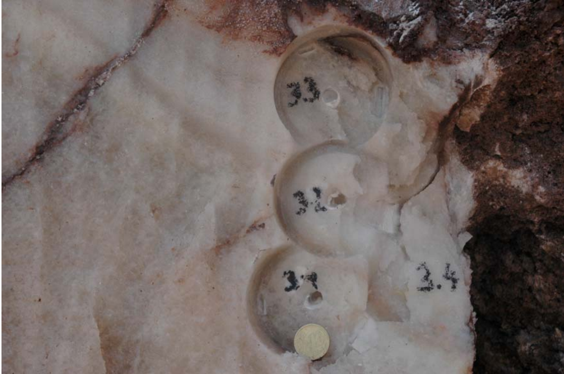
Fig. 3. Coarse-grained salt at the bottom of the image and thin layer of fine-grained salt at the top. The fine-grained layer is interpreted as a shear zone. Coin for scale.
