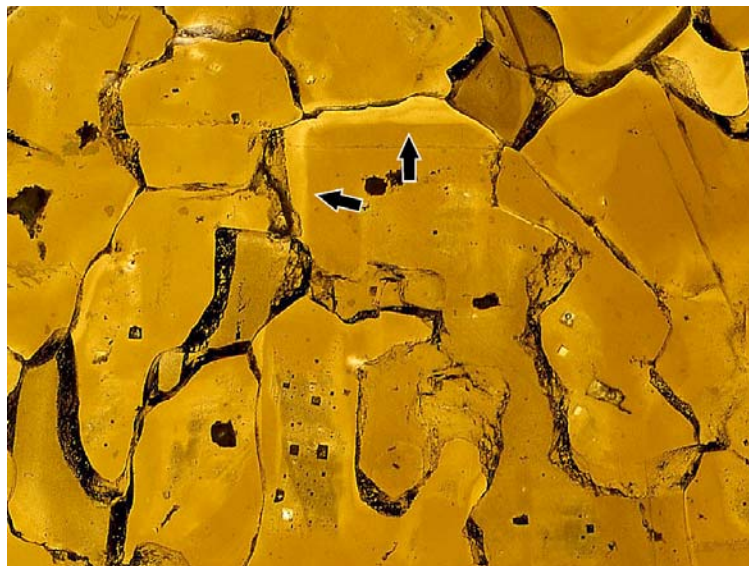
Fig. 13. Photomicrograph of sample gamma-irradiated at 35 °C from salt layer D (423.3 m). Minor grain boundary migration occurred in the grain in the middle of the image (see arrows), where the former (100) crystal face (grain boundary) migrated. The area swept by grain boundary migration is less colored. Grain boundaries occur as dark lines. Note that subgrain boundaries were not decorated with Na-precipitates by 35 °C irradiation. Note also that the thickness of the thin section is approximately 2 mm, so grain boundaries not perpendicular to the plane of image appear thicker. Plane polarized transmitted light image, image width is 2.4 cm.
