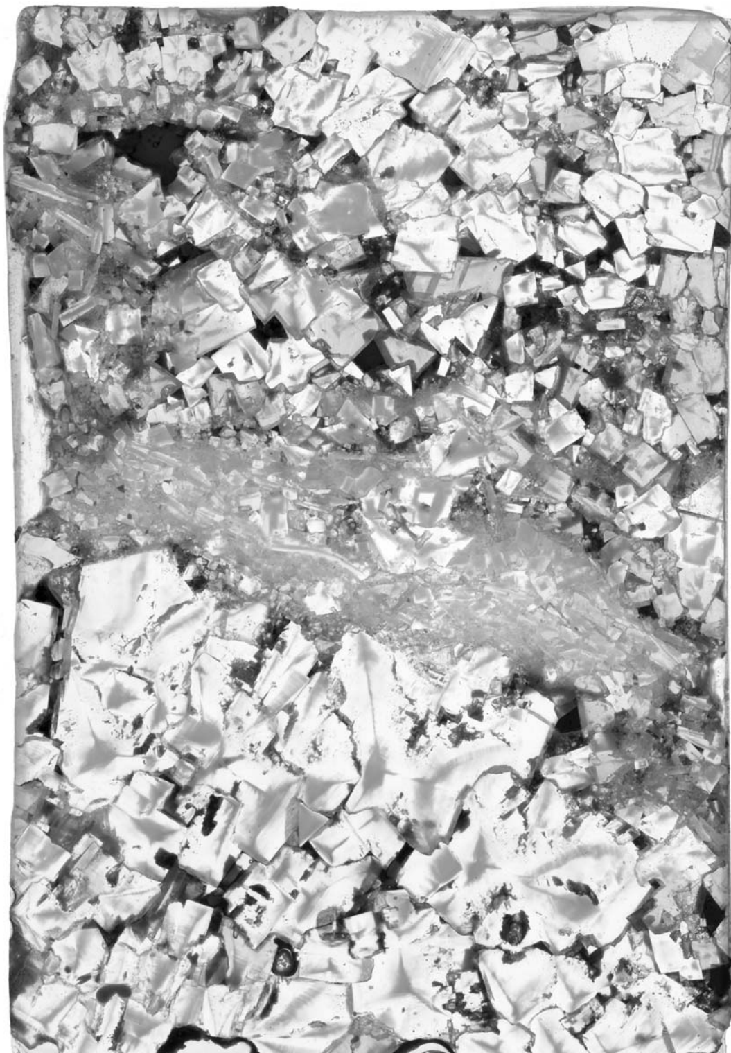
Fig. 3. Overview image of a thin section from a recent salt deposit from the Dead Sea (photographed in transmitted light). The sample is from a few meters of depth. Grain boundaries occur as dark curves; gray patches are fluid-inclusion-outlined chevrons and hoppers. The black areas between the grains are primary pores, which were filled with resin during sample preparation. In the middle of the image, a fine-grained layer of halite is visible. This layer is very likely consisting of sunken halite rafts. The coarse-grained part of this sample is an analogue for the Hengelo samples deposited in shallow-water environment. Image width is 4 cm.
