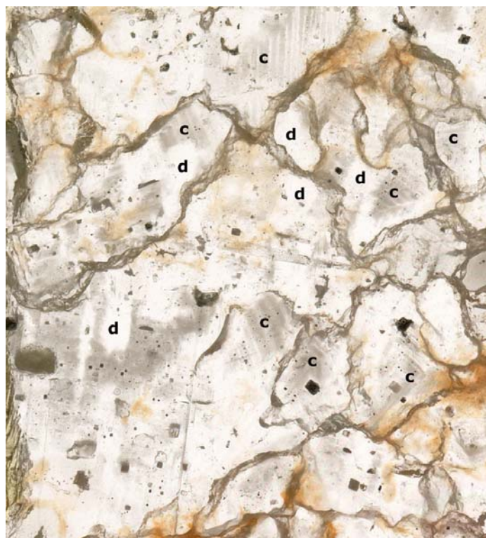
Fig. 4. Photomicrograph of an unirradiated sample (salt layer D, 423.3 m) showing primary fluid-inclusion-rich bands (c) and zones of clear halite (d). Clear halite commonly truncates fluid-inclusion-rich domains across sharp, curved, intracrystalline boundaries. Grain boundaries show up as dark curves in thin section. Secondary phases occurring at grain boundaries are anhydrite and polyhalite. Transmitted light image, image width is 2 cm.
