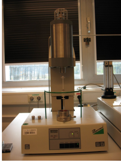
Figure 2.5: Picture of the High-Temperature Differential Scanning Calorimeter DSC 404C by Netzsch.
