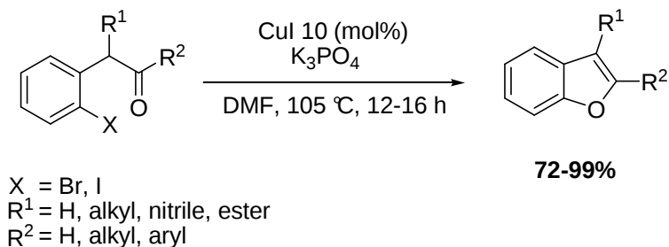
Scheme 39. CuI-catalyzed intramolecular C-O cross-coupling by Dormer.
