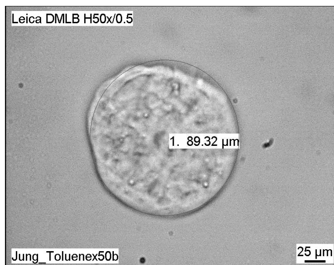
Figure 4. Micrography of the appearance of crosslinked polystyrene suspension in toluene.
