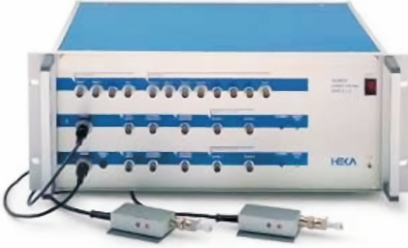
Figure 3.6: Photograph of the EPC 9 double patch-clamp amplifier and two preamplification head-stages. The main amplifier provided several in- and out-puts to e.g. control a perfusion system or acquire FET or MEA signals in parallel to patch-clamp recordings. All functions were controlled by the software TIDA .
