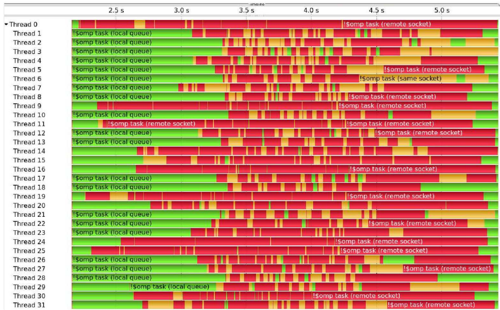
Figure 5.13: Vampir screenshot showing the tasks during the execution of the load balancing benchmark with the GNU runtime system. Tasks executed on the creating thread are shown in green, stolen tasks from the same NUMA-node in orange and from remote NUMA-nodes in red. Comparing this figure to figure 5.12, a huge difference in the way tasks are scheduled in the GNU and Intel runtime can be observed.
